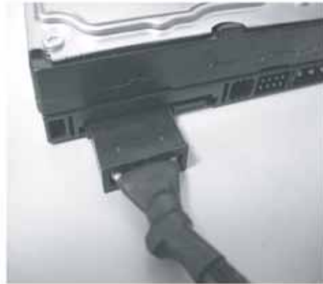
SATA connectors used for SATA Hard Drives.
