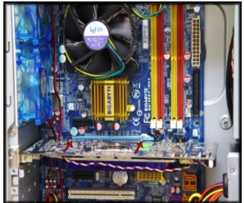
3.1 Remove the metal PCI slot cover(s) from the slots to be used and install devices into their respective slots. (i.e. x1, x8, x16, etc.)
