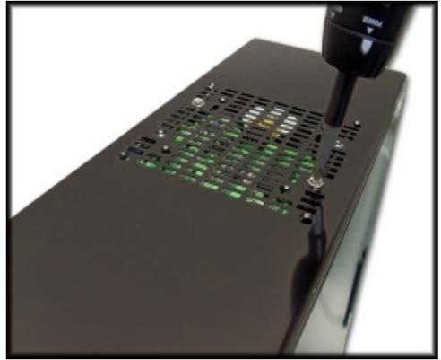
6.1 The X-Master gives you the option of installing additional devices. (up to 2 x 80 or 120mm fans, or 2 hard drives.) Mount device to area of your choice and screw to case. (If adding a case fan to the lower area, chassis should be laid on its side so as not to impede airflow.)
