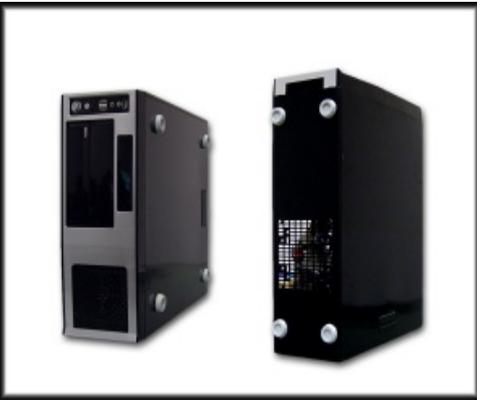
7.1 Mount case feet to the chassis. You have the choice of standing the chassis upright (tower) and mounting the case feet to the bottom, or laying the chassis on the non-vented side and mounting them. (desktop style)
