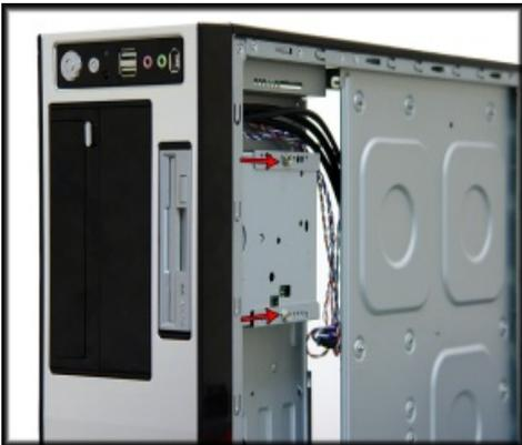
2.7 If installing a 3½" device that needs to be accessible from the front panel, you will need to place the device into the preferred position, then screw to case.
