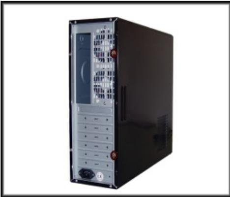
1.1 Remove thumbscrews from the rear of the chassis.
