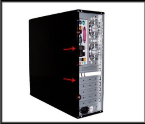
2.5 Remove the right-side panel. Extract the two rear screws and slide the panel outward to release.
