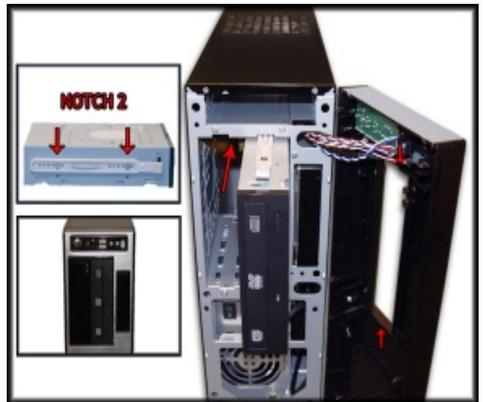
2.4 Remove the front panel drive bay cover. Remove the 'drive-rail pins' and remount into notch #2. Mount rails to the sides to the optical drive and install.
