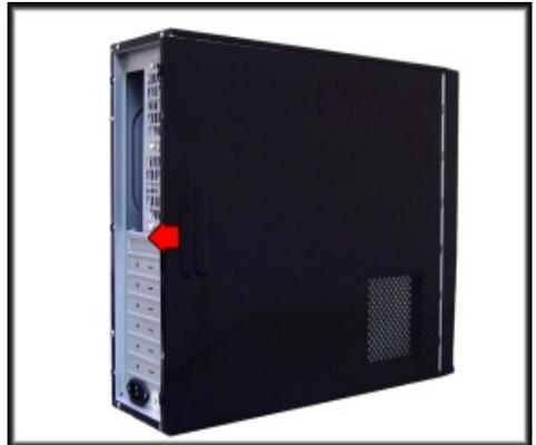
1.2 Remove left-side panel from case by sliding it in the direction shown.
