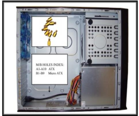
1.4 For standoff screw placement, follow the M/B Holes Index which is engraved onto the motherboard tray. Full ATX boards (9.6" x 12") will use notches A1-A10. Full Micro ATX boards (9.6" x 9.6") will use B1-B9.
