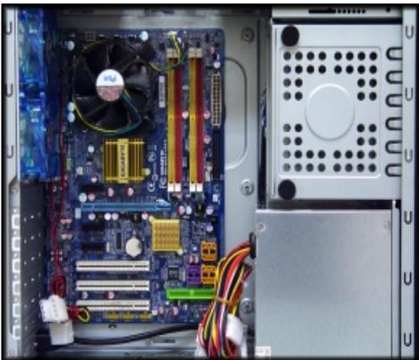
1.5 Align motherboard over the standoff screws and secure to the case using the included mounting hardware.
