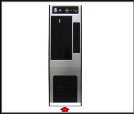
2.1 In order to install optical and hard-disk drives, you will 1st need to re-move the front panel. Get a solid grip on the vent at the bottom of the panel and pull firmly.
