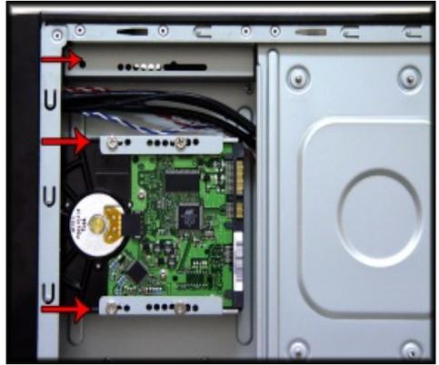
2.6 Install hard-drive(s) into the side and /or upper 3½" drive bay(s) and secure to the case.
