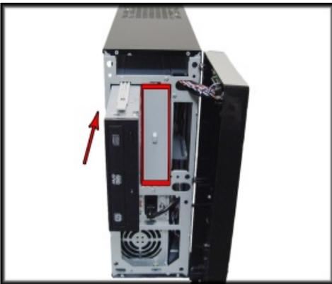
2.3 Align rails with drive bay and insert. Drive will sit behind the drive cover, and can be activated by pressing the button located on the cover. If installing a 2nd optical drive, also remove the metal shield from drive bay.
